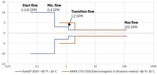
Note: At flows between 'Start flow' and 'Maximum flow' measurement occurs – however the accuracy is only guaranteed in the range from minimum flow to maximum flow
